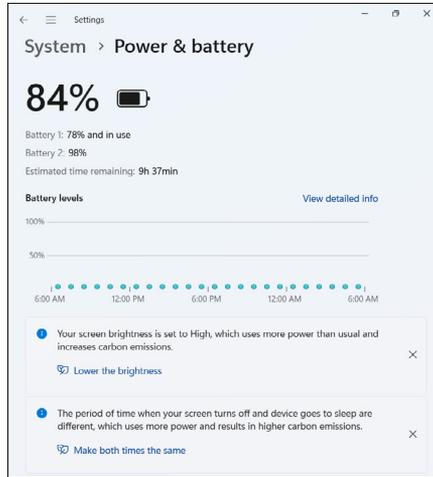
If the Mesa 4 battery reaches a very low charge, the tablet hibernates to prevent further drain on the battery. To exit hibernation, charge the battery until the charge is sufficient to power the tablet. Then, press the power button.
