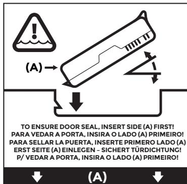
3. Rotate the tabbed edge down until the battery sits flat in the compartment.
